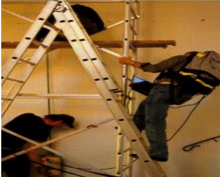
Fig. 6. The Great Pyramid. GPR research project in the "King's Chamber". Folding ladder (up to 4 m) for making vertical GPR section lines
