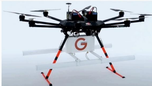
Fig. 20. MALA GEODrone 80 system - with GPR 80 MHz antennas placed on a drone-type flying system
